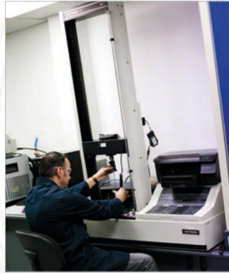
Tensometer Testing a range of tensile related properties, including tensile strength, elongation and tear strength.
