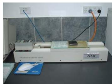
Coefficient of Friction Tester
