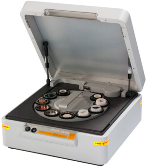
XRF Analyser (X-Ray Fluorescence) Used for testing curative levels in elastomers.
