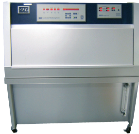
QUV Weatherometer This equipment accelerates the effects of sunlight, rain and condensation.
