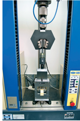
Tensometer Used for testing a range of tensile related properties, including tensile strength, elongation and tear strength.
